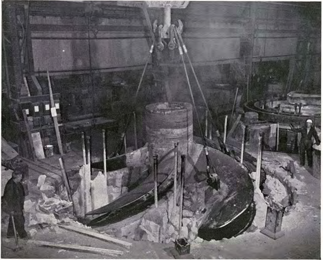
The breaking out of a typical large propeller from its mould.
